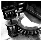
PHOTOGRAPHS DEVICE FOR GRINDING CONCAVE MIRRORS LEONARDO DA VINCI
